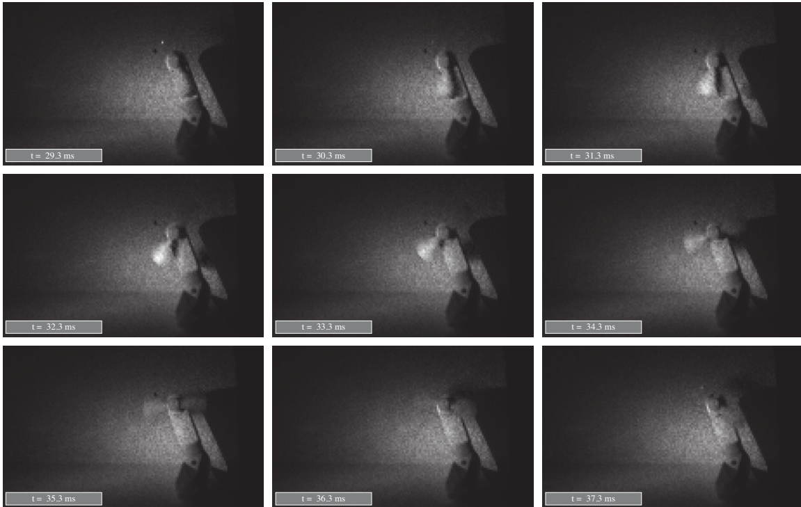
Figure 4.5.9: Images show various stages of a fan spinning, rendered at 1 kfps.
