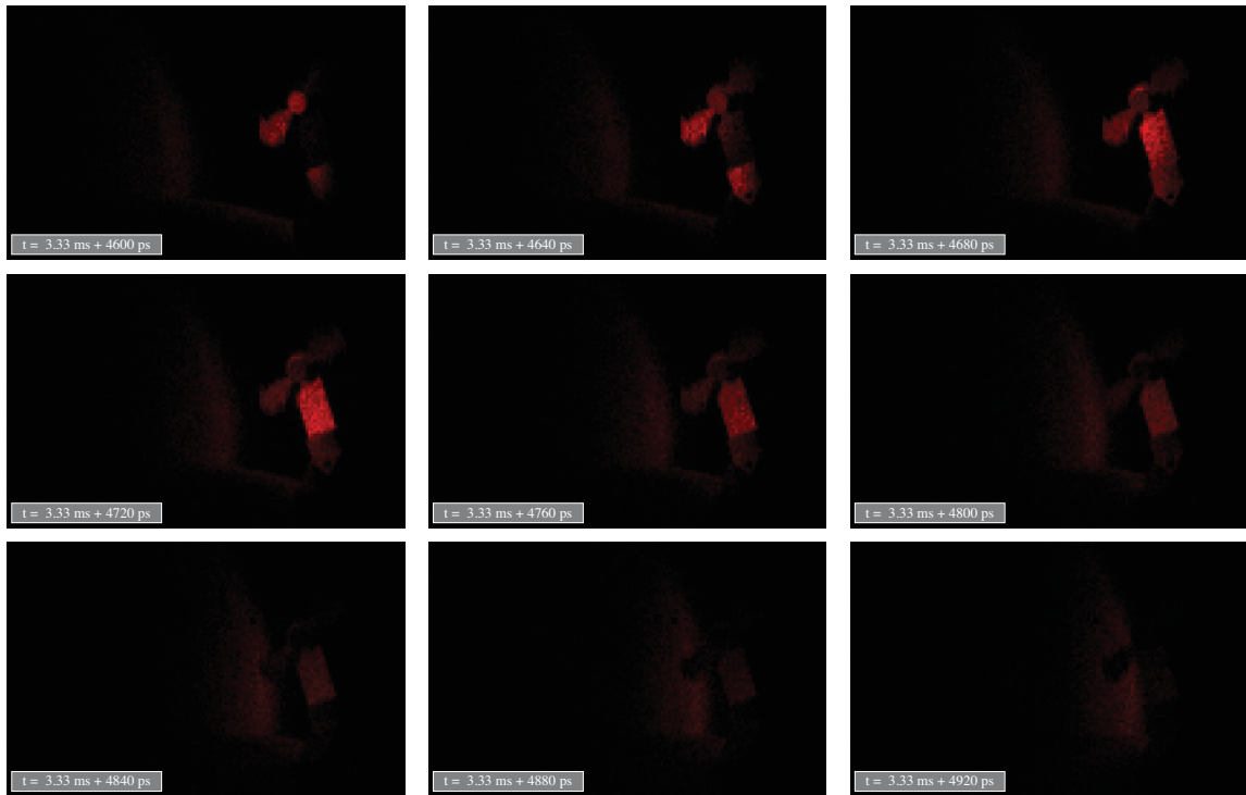
Figure 4.5.14: Color images depicting the propagation of a picosecond laser pulse across two planes and a fan. At this timescale, only the red pulsed laser contributes to the illumination of the scene.
