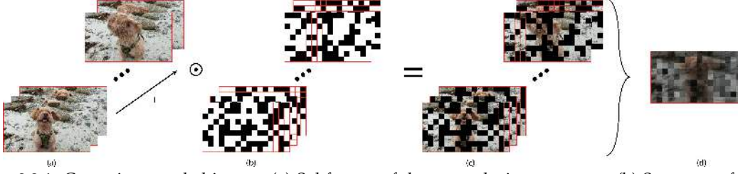
Figure 2.3.1: Capturing a coded image. (a) Subframes of the scene during exposure. (b) Sequence of codes used during exposure; each code lasts for one subframe. (c) The codes block specific pixels from collecting light during each subframe so the camera sees a partly obscured view of the scene. (d) Coded image output at the end of the exposure.
