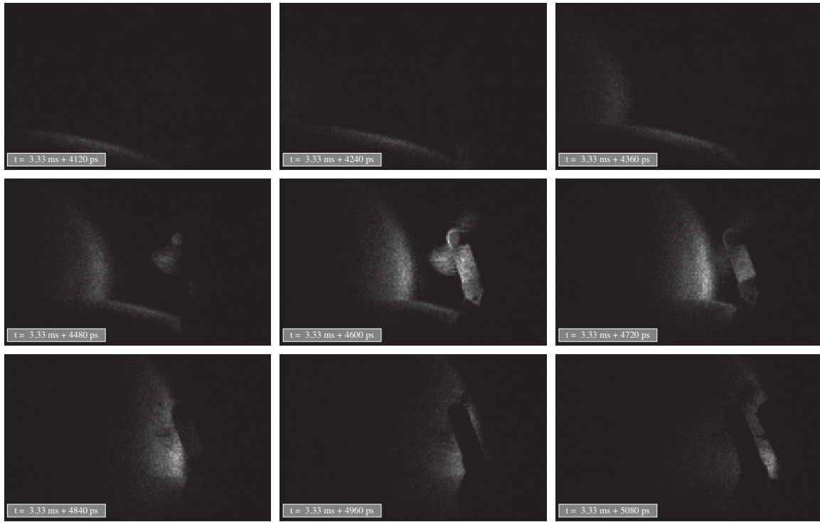
Figure 4.5.10: Images show a picosecond laser pulse propagating over two planes and a fan. Note how the fan blades appear as frozen. The effective frame rate is 250 Gfps.
