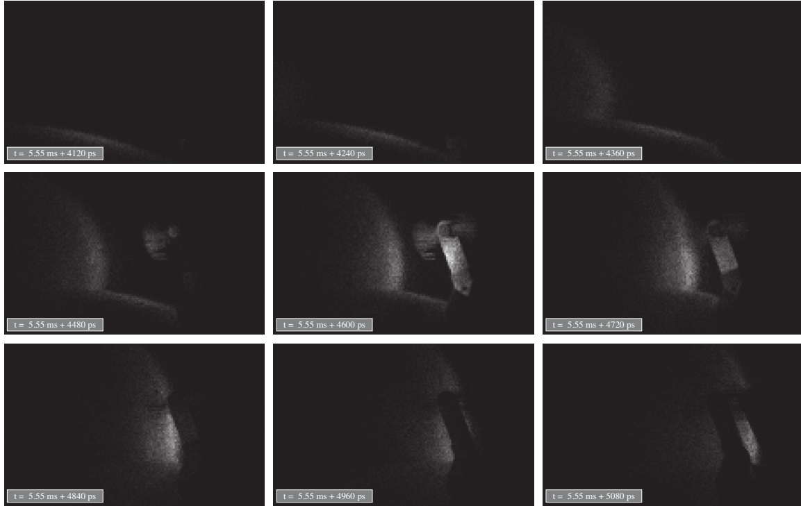
Figure 4.5.12: Images show a picosecond laser pulse propagating over two planes and a fan. The fan blades are at a different position demonstrating the unique capability of our approach to freeze time at all timescales .
